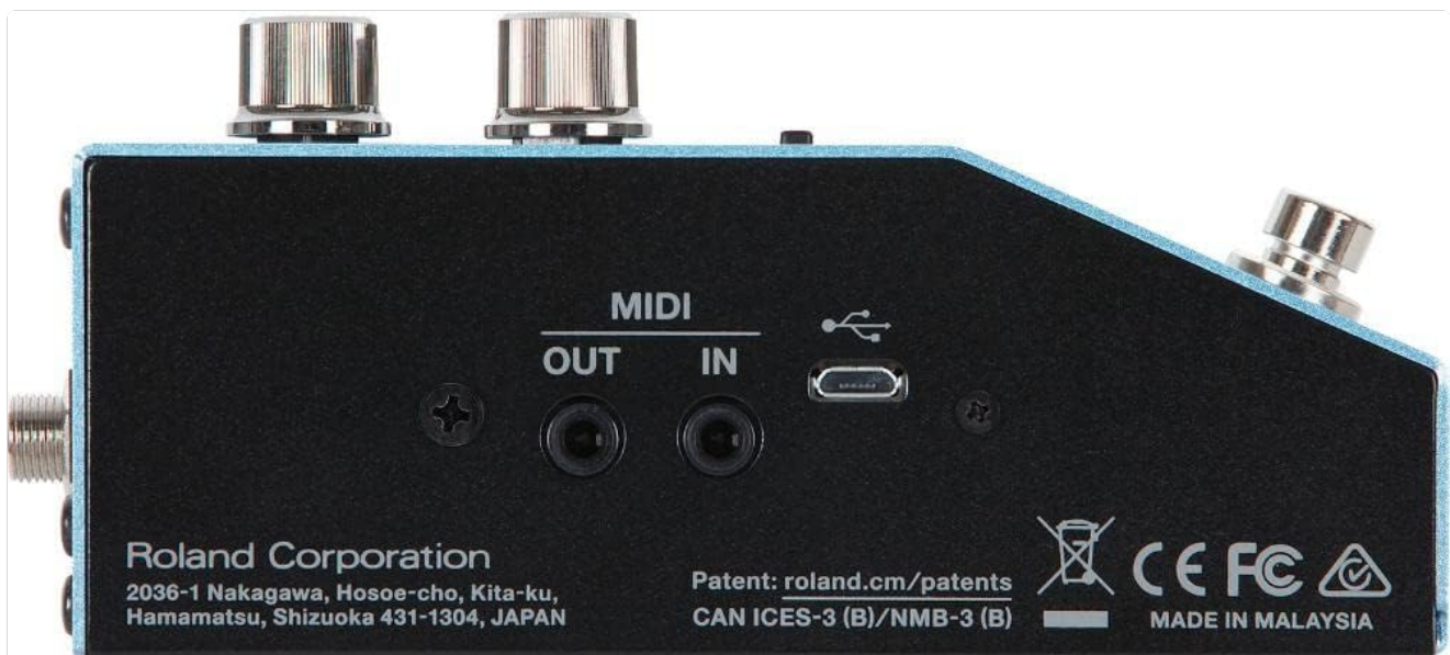
Figure 3: Side Panel Connections of the MD-200. This image shows the side of the pedal with the MIDI IN, MIDI OUT, and USB
