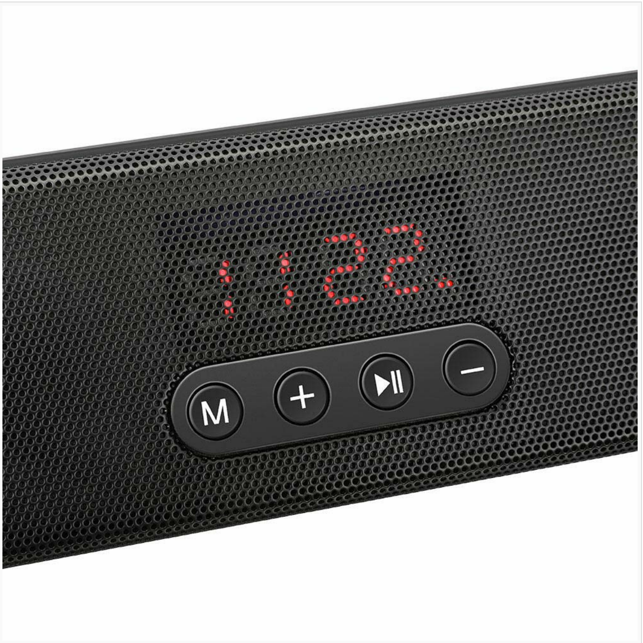
Figure 3.3: Close-up view of the control panel, showing the 'M' (Mode), '+' (Volume Up/Next Track), Play/Pause, and '-' (Volume Down/Previous Track) buttons.
