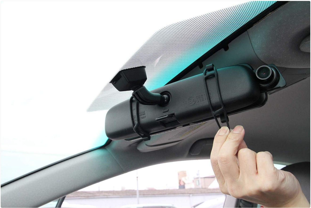
Figure 4: Attaching the drive recorder mirror to the existing rearview mirror using straps.
