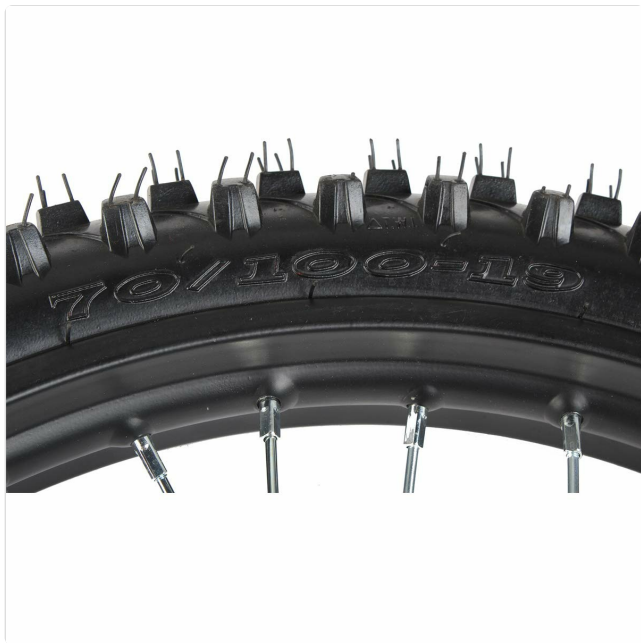
Figure 3: Close-up of the tire sidewall showing the 70/100-19 size marking.
