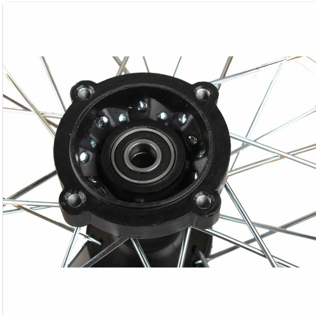
Figure 4: Detail of the wheel hub, showing the integrated 15mm bearing assembly.
