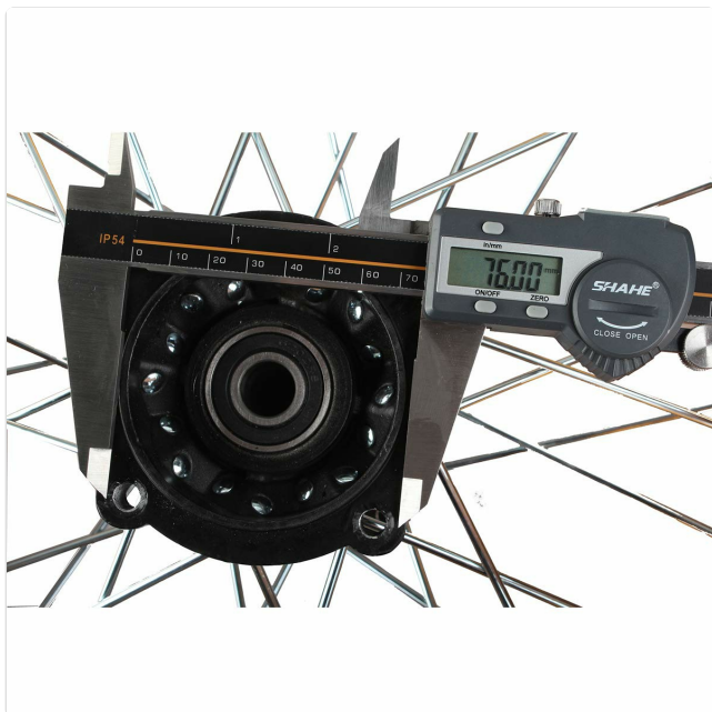
Figure 6: Digital caliper measuring the brake rotor inner diameter at 76mm.
