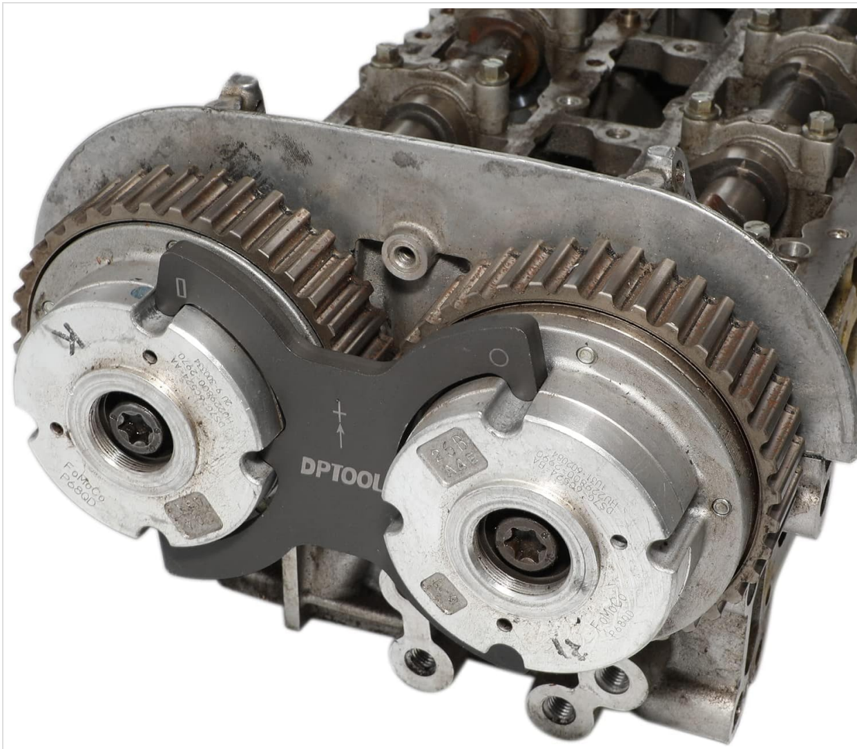
Image 5.4: The camshaft sprocket locking tool (e.g., OEM 303-1097) correctly positioned to secure the camshaft sprockets.
