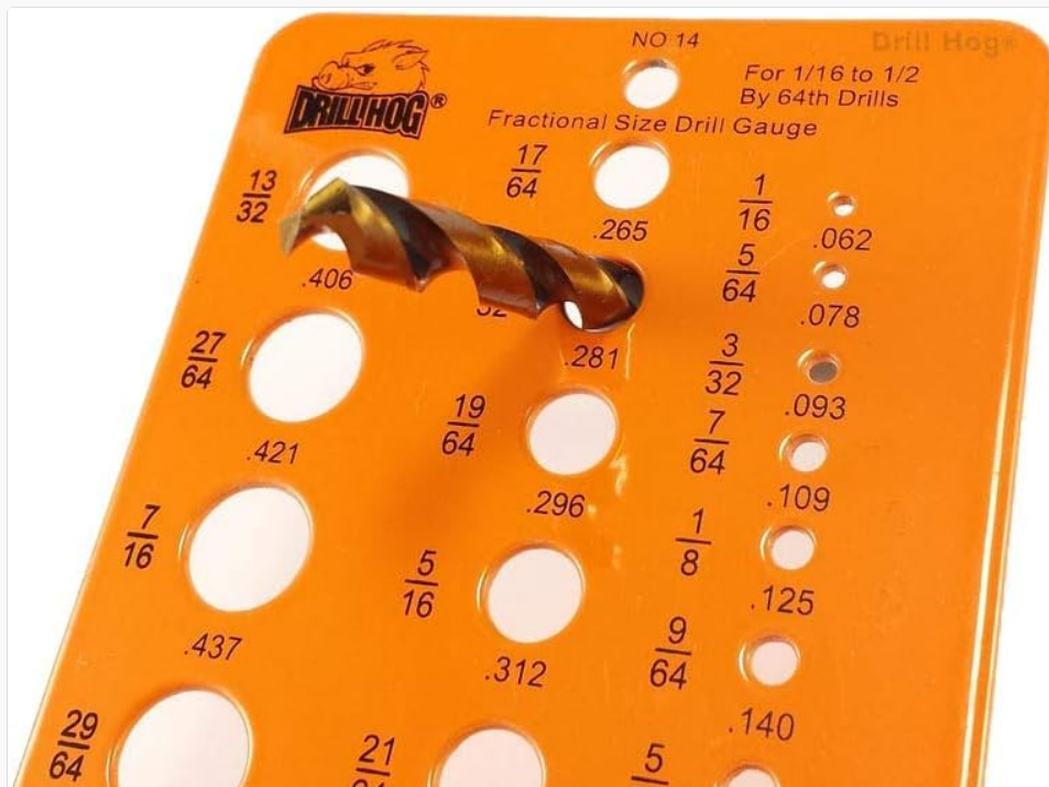
Image 1: A drill bit being measured using the Drill Hog Drill Gauge. The bit fits snugly into the designated hole, indicating its precise size.
