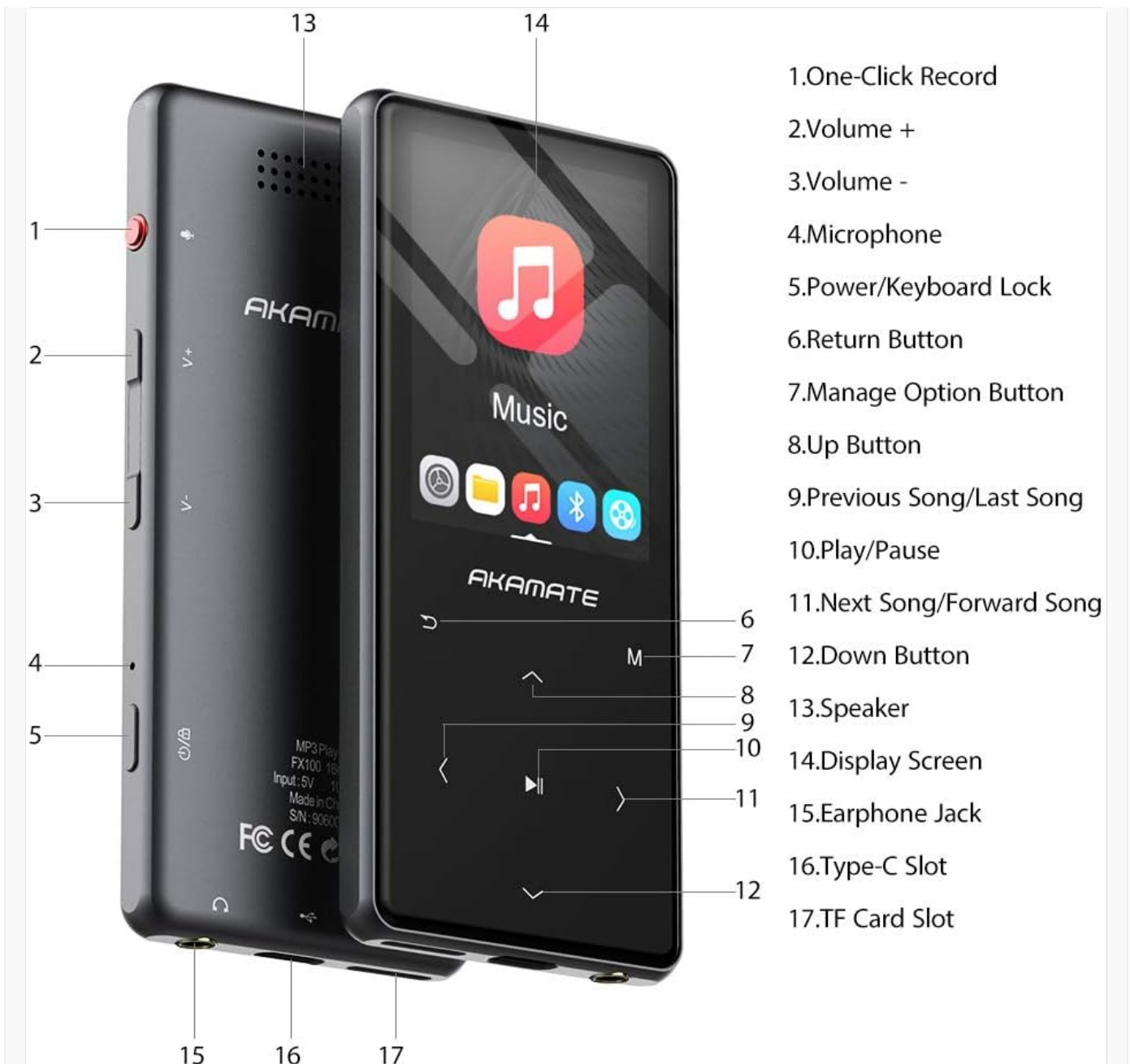
Figure 4.1: Detailed diagram of the AKAMATE FX100 MP3 Player's physical features and controls.
