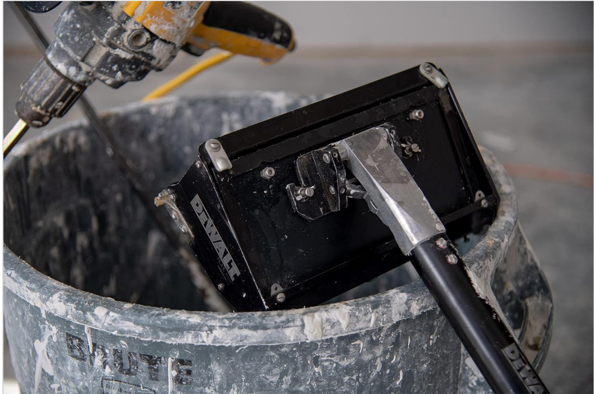
Image 3: The flat box and extension handle being cleaned in a bucket after use.
