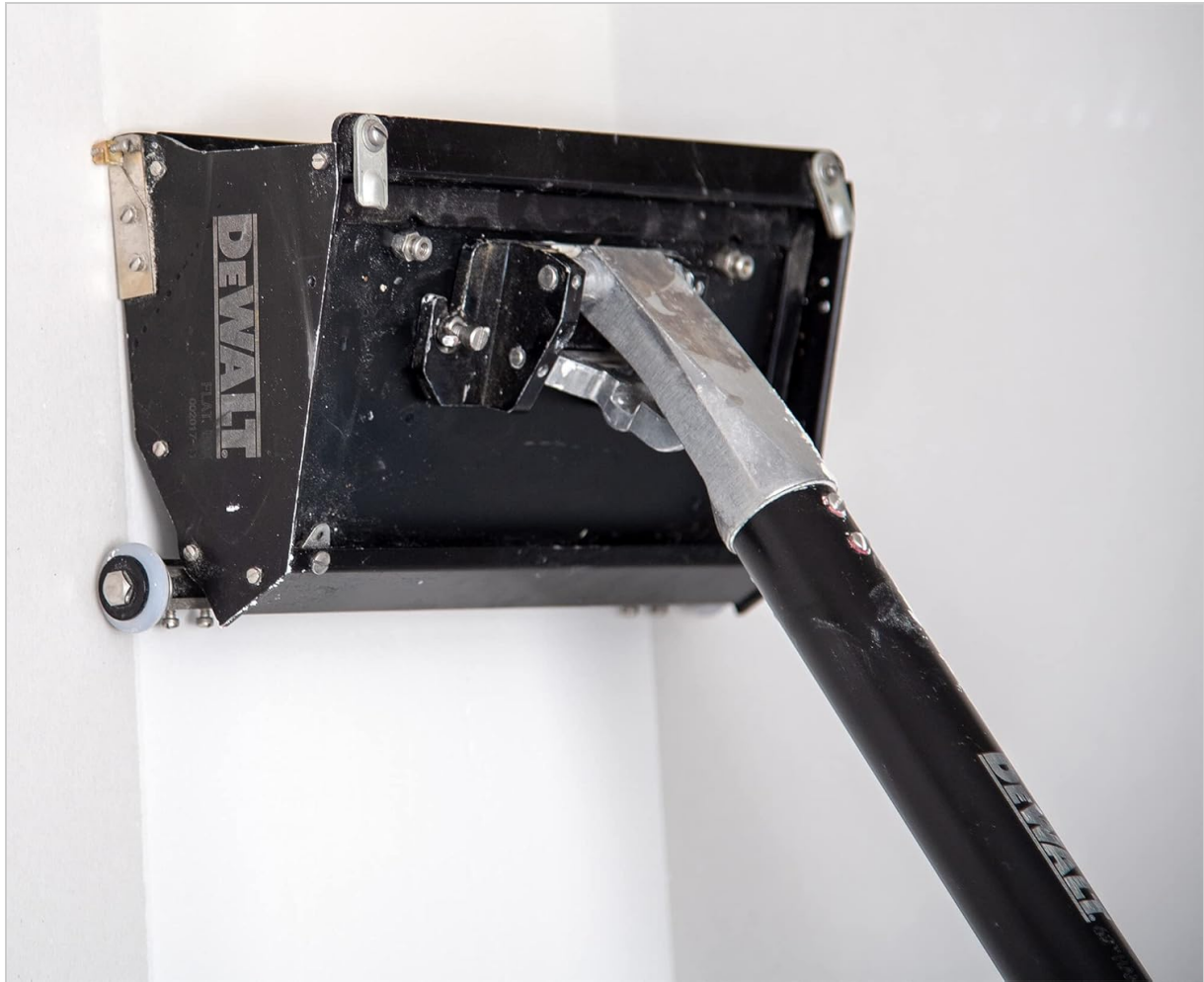
Image 1: The DEWALT Flat Box Extension Handle connected to a flat box, ready for use on a drywall seam.
