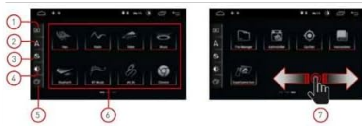
Image 4.2: Diagram illustrating the screen layout with numbered side buttons (1-4), main application area (6), and the swipe gesture (7) for navigating between screens. Element 5 points to the bottom navigation bar.
