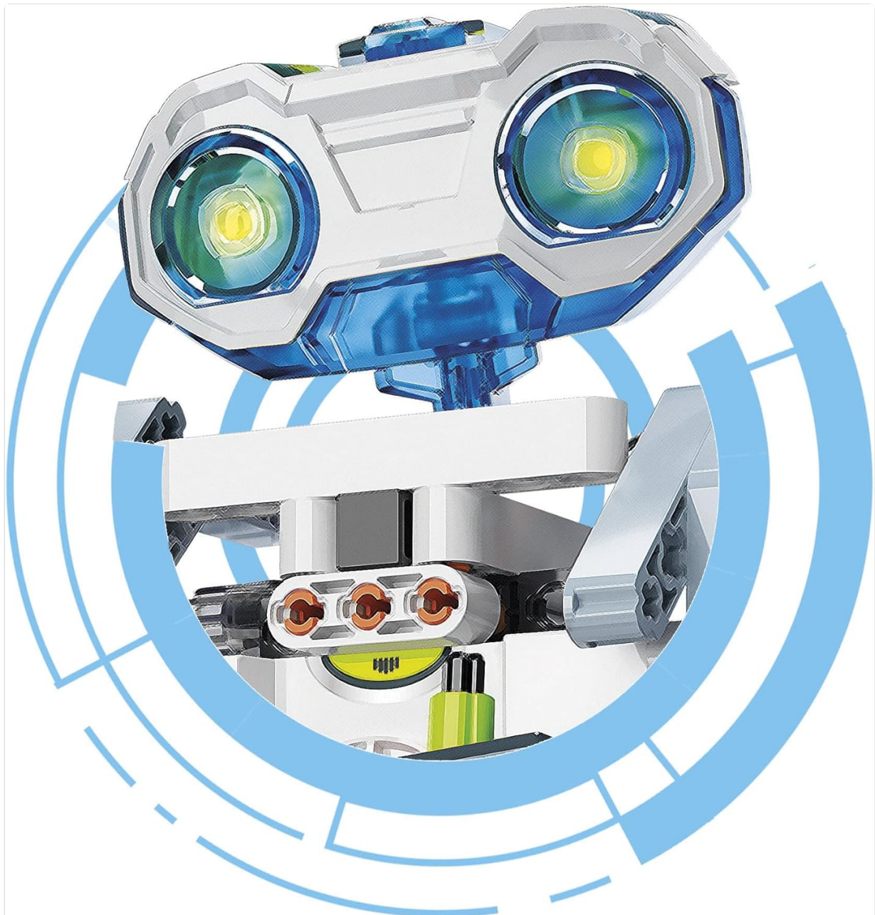
Figure 6.1: A detailed view of the robot's head, highlighting the eyes (LEDs) and the infrared sensor module for environmental interaction.
