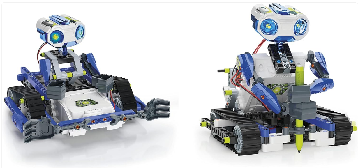
Figure 4.2: The X1-Drawer robot (left) designed for drawing, and the X2-Elevator robot (right) configured for lifting or pushing objects.
