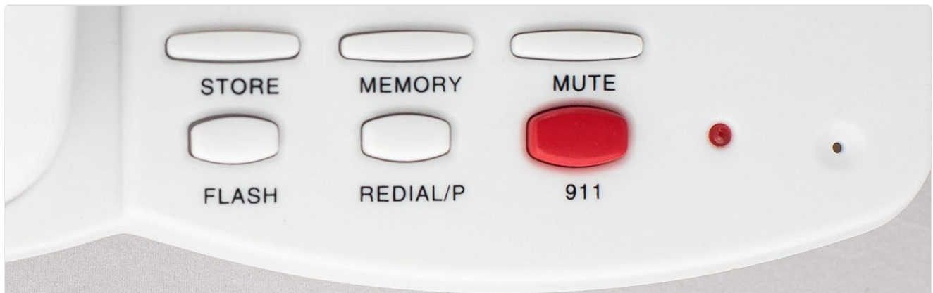
Figure 3: Close-up view of the control buttons, including STORE, MEMORY, MUTE, FLASH, REDIAL/P, and the red 911 button. These buttons are used for various calling functions and memory programming.
