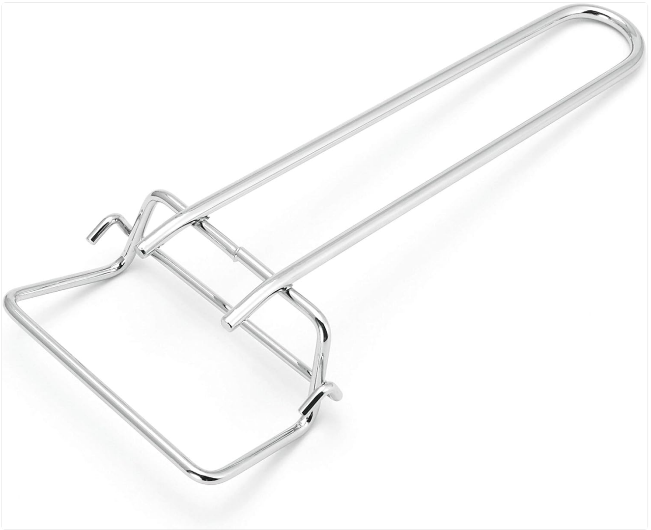
Figure 4: Tongs. Metal tongs for safely gripping and removing hot trays or racks from the oven.
