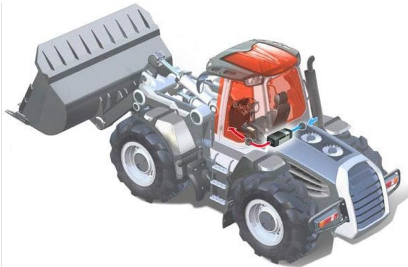
Figure 5.2: Illustrative diagram of a Webasto heater installed in a loader vehicle, indicating the heater unit's position and the distribution of heated air within the cabin.
