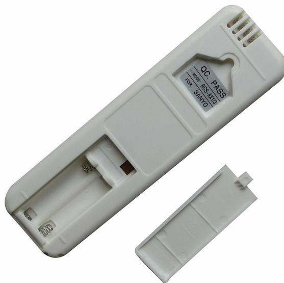
Figure 3.3: Battery compartment with cover removed.
