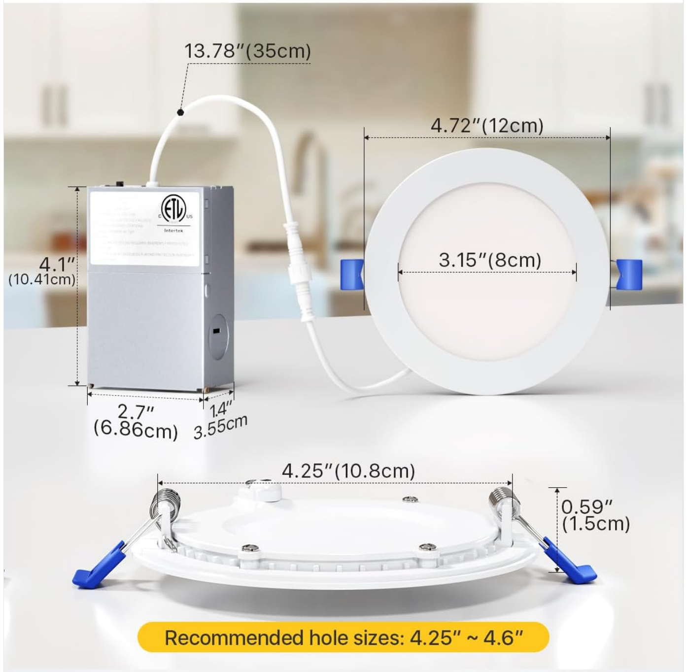
Image 2: Detailed dimensions of the Ensenior 4-inch LED Recessed Light and its junction box.
