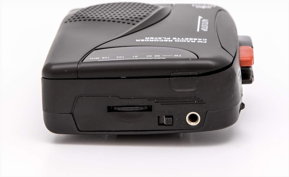
Figure 1: Side View. This image displays the side of the cassette player, highlighting the volume control wheel, the 3.5mm headphone jack, and the 3V DC-in port for external power.
