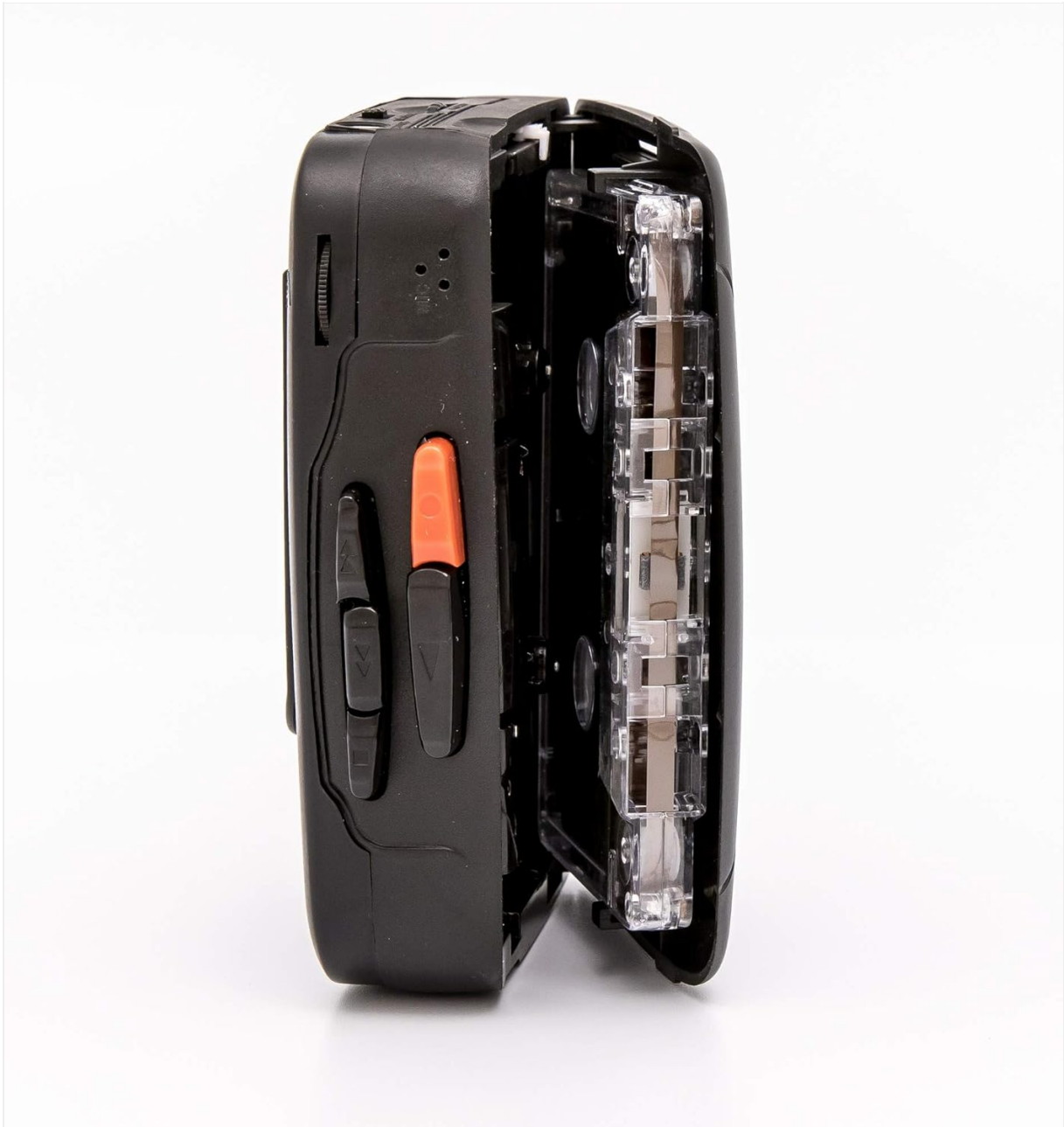
Figure 4: Cassette Compartment. This image shows the cassette compartment open with a tape correctly inserted, ready for playback or recording.
