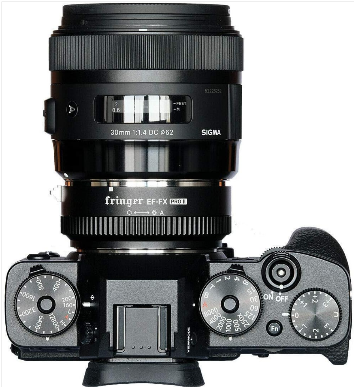
Figure 3.3: Top view of a Fujifilm camera with the Fringer EF-FX PRO II adapter and a Sigma 30mm lens mounted.
