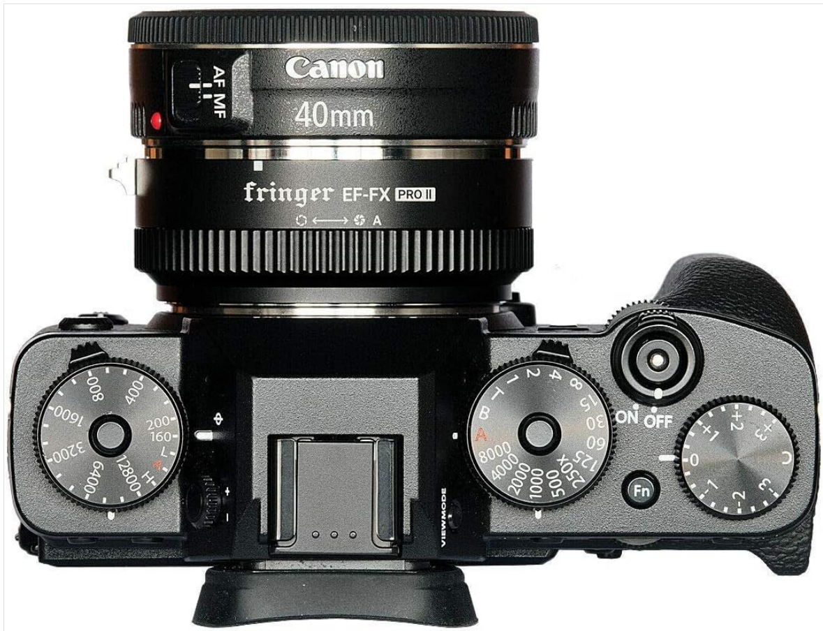
Figure 3.2: Top view of a Fujifilm camera with the Fringer EF-FX PRO II adapter and a Canon 40mm lens mounted.
