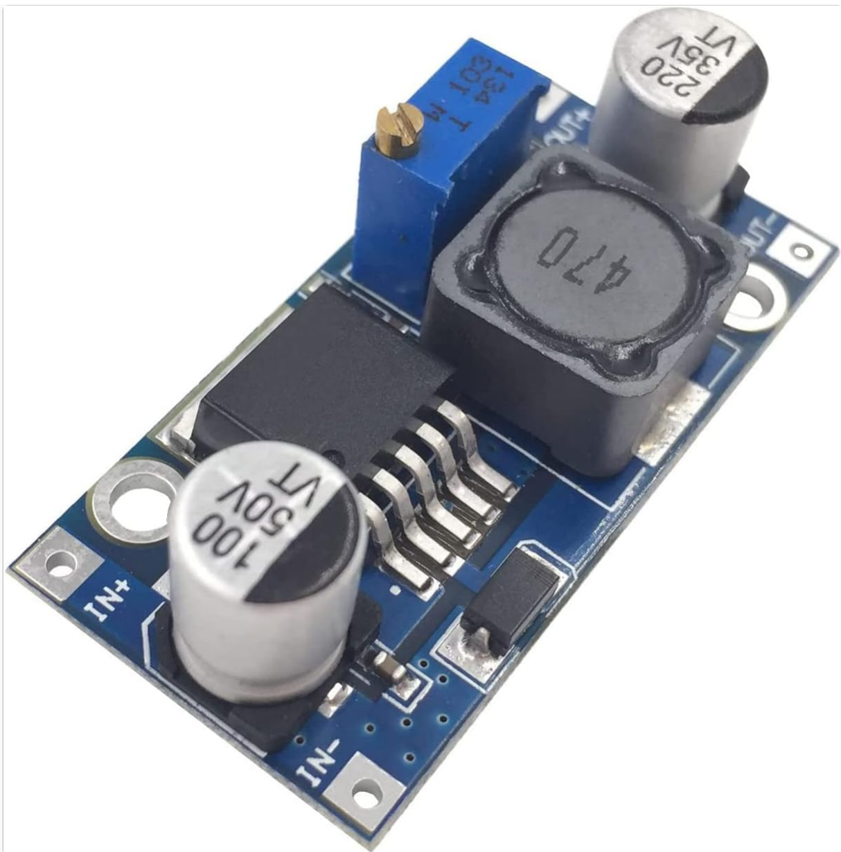
Figure 1: Top view of the Valefod LM2596 DC-DC Buck Converter module, showing the input/output terminals, potentiometer, inductor, and capacitors.
