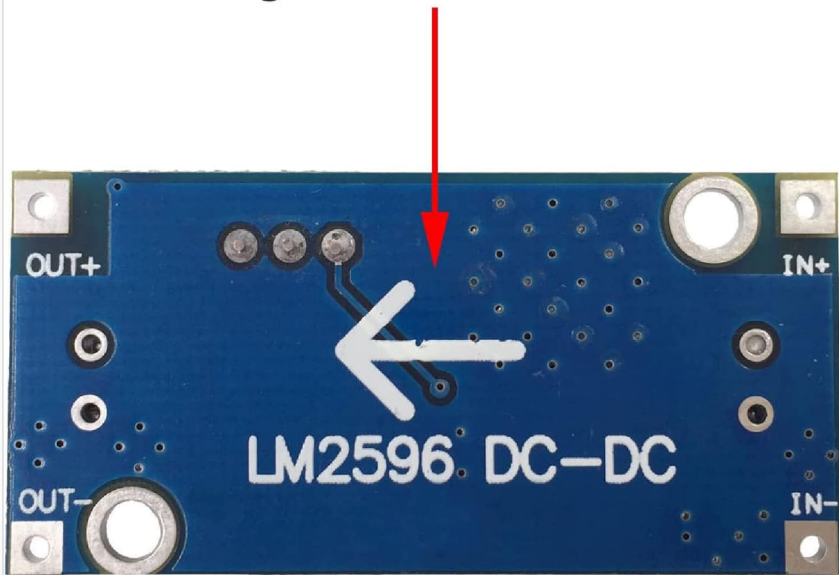
Figure 2: Bottom view of the LM2596 DC-DC module, indicating the current flow direction and model number.
