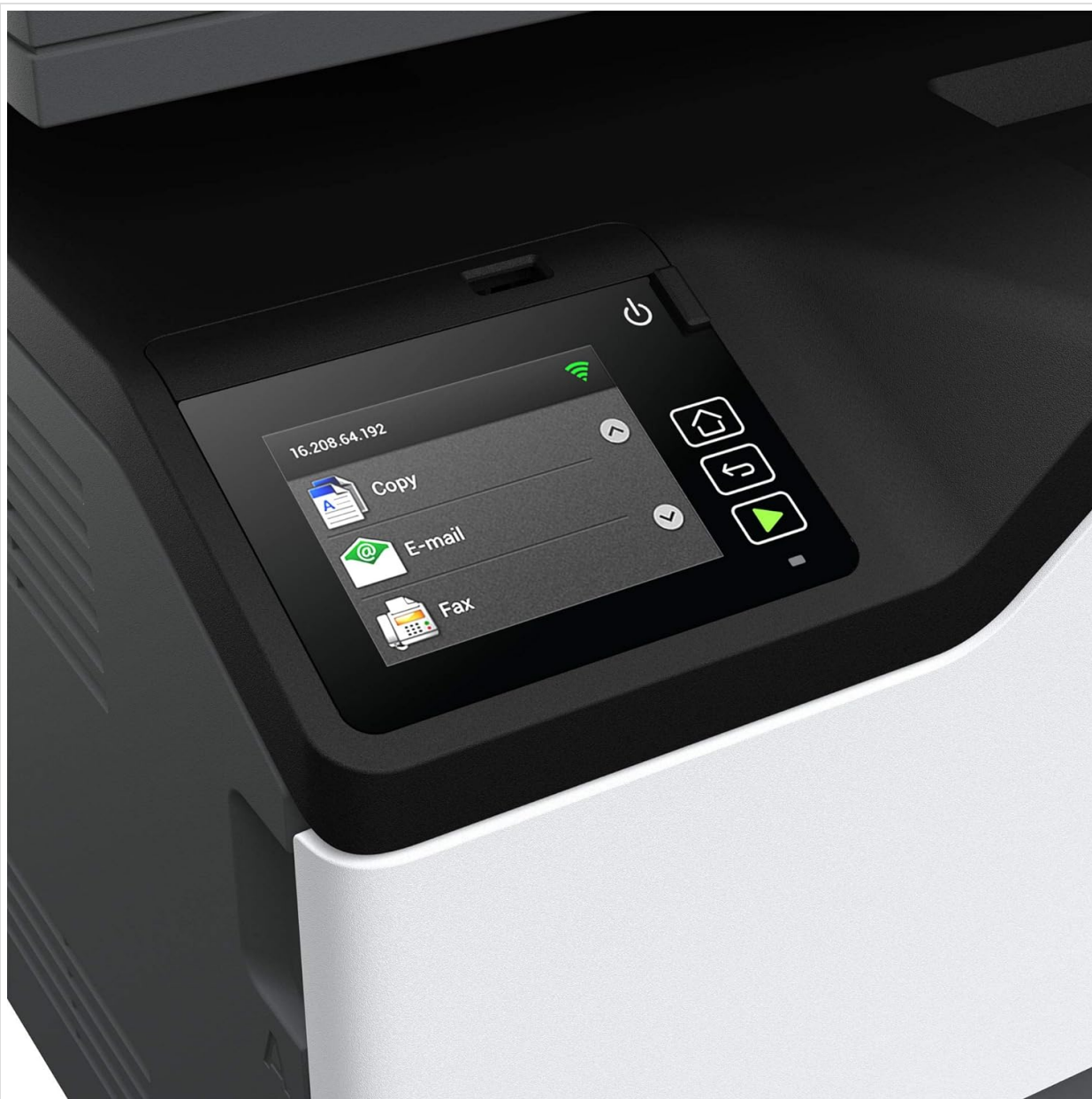
Figure 2.1: Printer control panel with touch screen.
