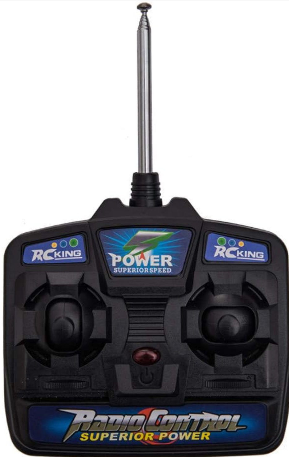
Figure 1: Front view of the SHENGLE 27MHz Remote Control Transmitter, showing two joysticks and an antenna.
