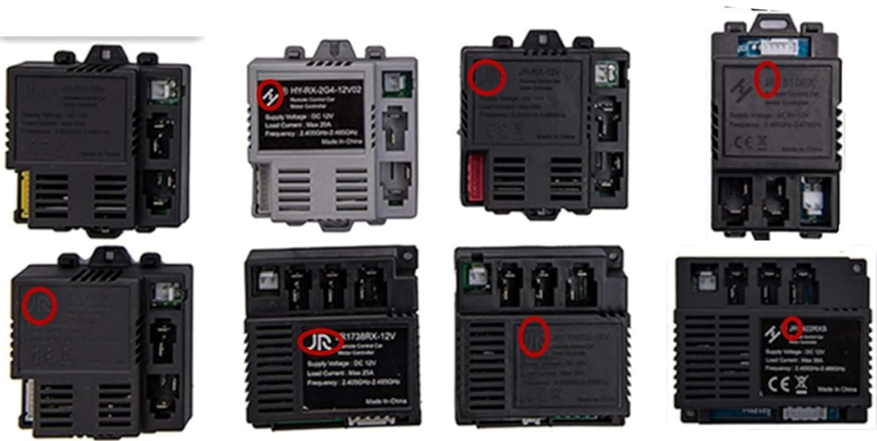
Figure 4: The 27MHz remote control is not compatible with 2.4G receivers, as illustrated with several incompatible receiver types.
