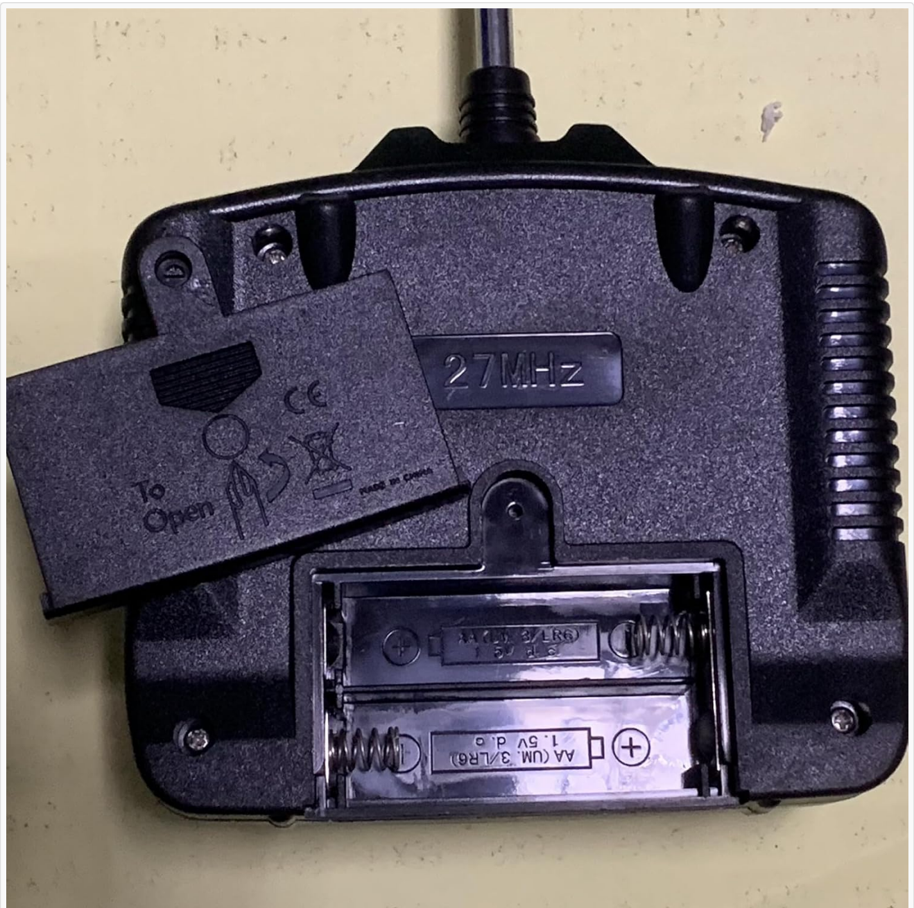
Figure 2: Back of the remote control with the battery compartment open, illustrating battery placement.
