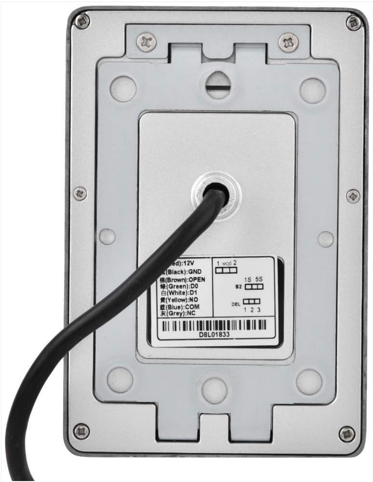
Figure 7: Rear view of the access control reader with wiring terminals. Reference number: D8L01833.
