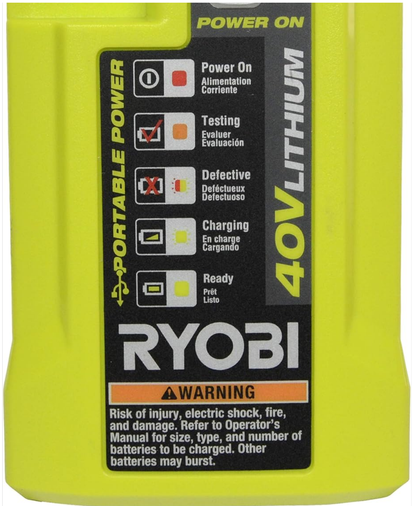
Figure 4: Close-up view of the RYOBI OP404 charger's LED indicators, detailing various status lights.
