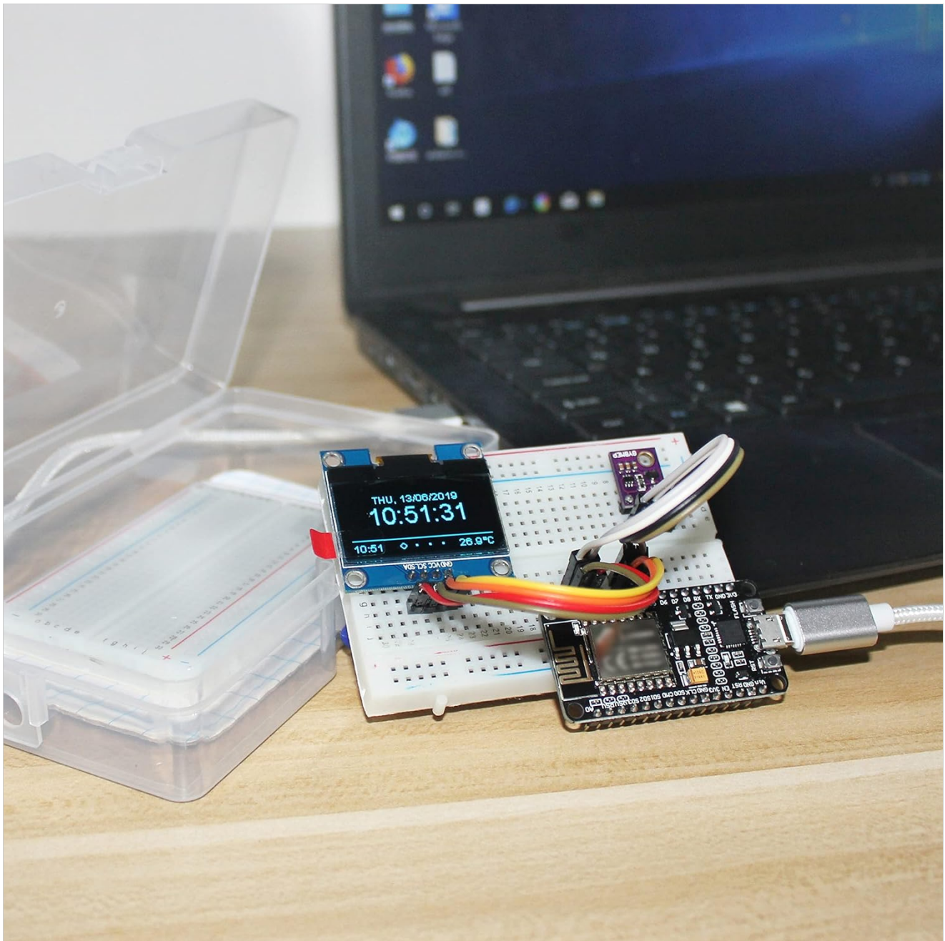
Image: The assembled WiFi Weather Station Kit on a breadboard, connected to a laptop for programming.
