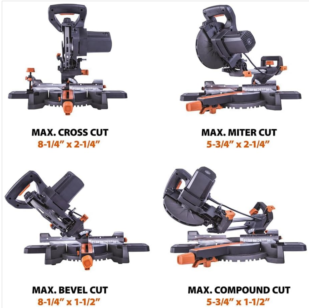
Figure 3.1: Visual guide to maximum cutting capacities for various cut types: cross, miter, bevel, and compound.
