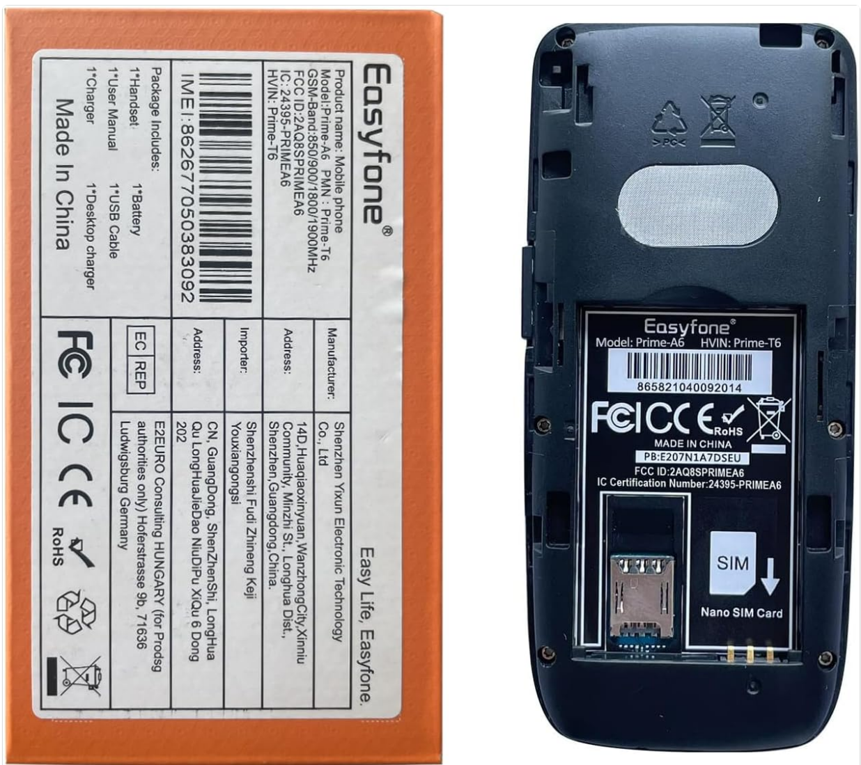
The back of the Easyfone Prime-T6 phone with the cover removed, showing the SIM card slot and battery compartment.
