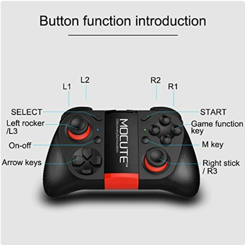
Figure 4.1: Detailed diagram illustrating the function of each button and control on the MOCUTE 050 gamepad, including L1, L2, R1, R2, SELECT, START, Left/Right Rockers (L3/R3), Arrow Keys, Game Function Keys, and M key.
