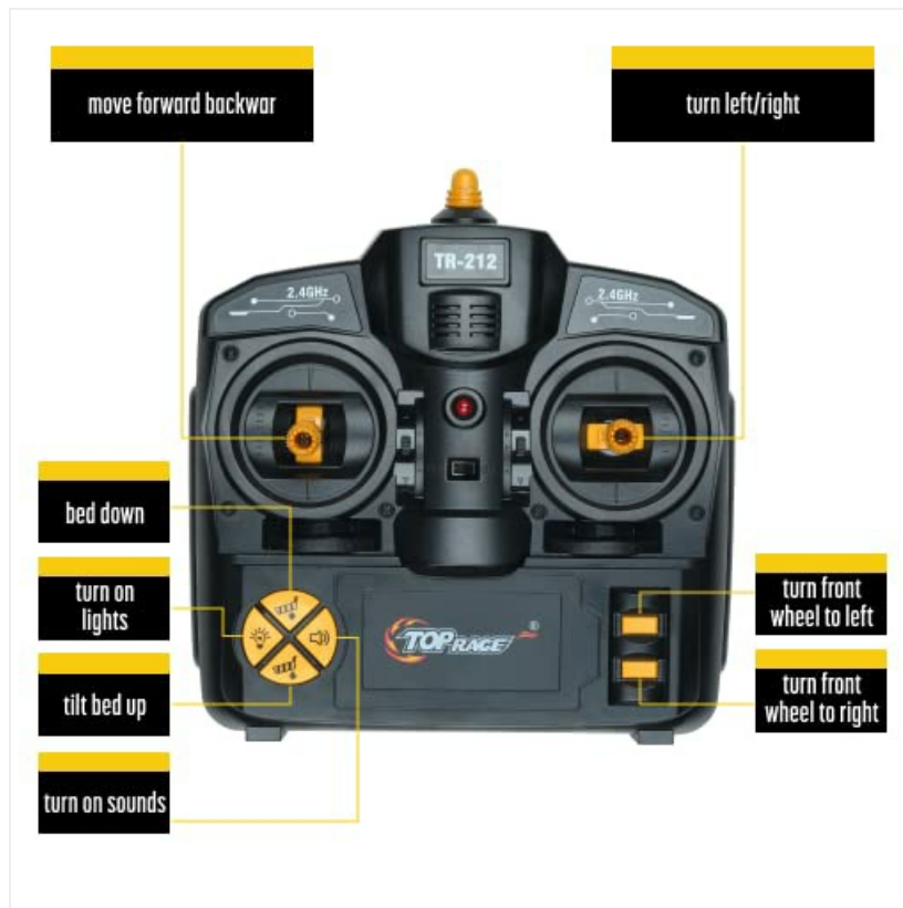
Image: Diagram of the Top Race TR-212 remote control, showing labels for moving forward/backward, turning left/right, bed up/down, turning lights on, and turning sounds on.
