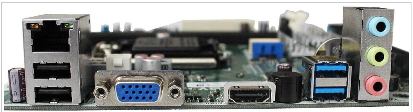
Figure 4: Rear I/O panel of the IPM81-SV REV:1.01 motherboard, showing ports for Ethernet, VGA, HDMI, USB 2.0, USB 3.0, and audio jacks.
