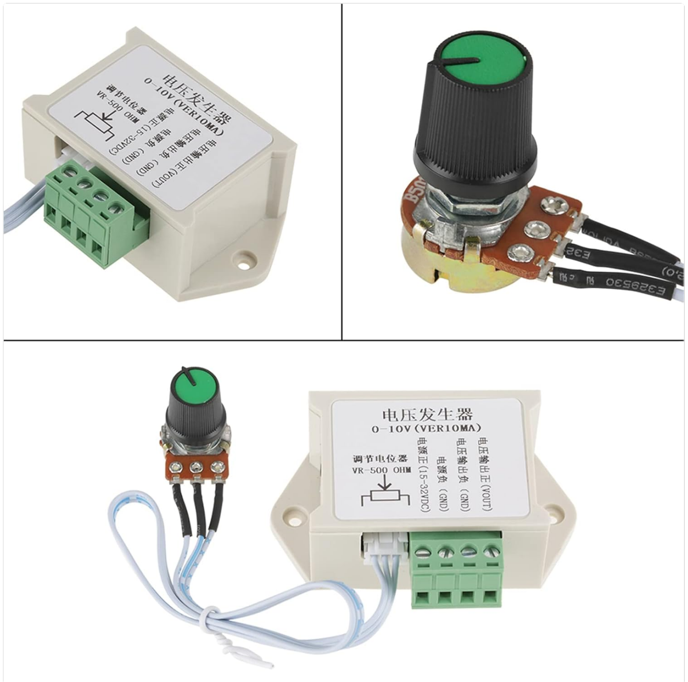
Figure 5.1: Adjusting the output voltage with the potentiometer.
