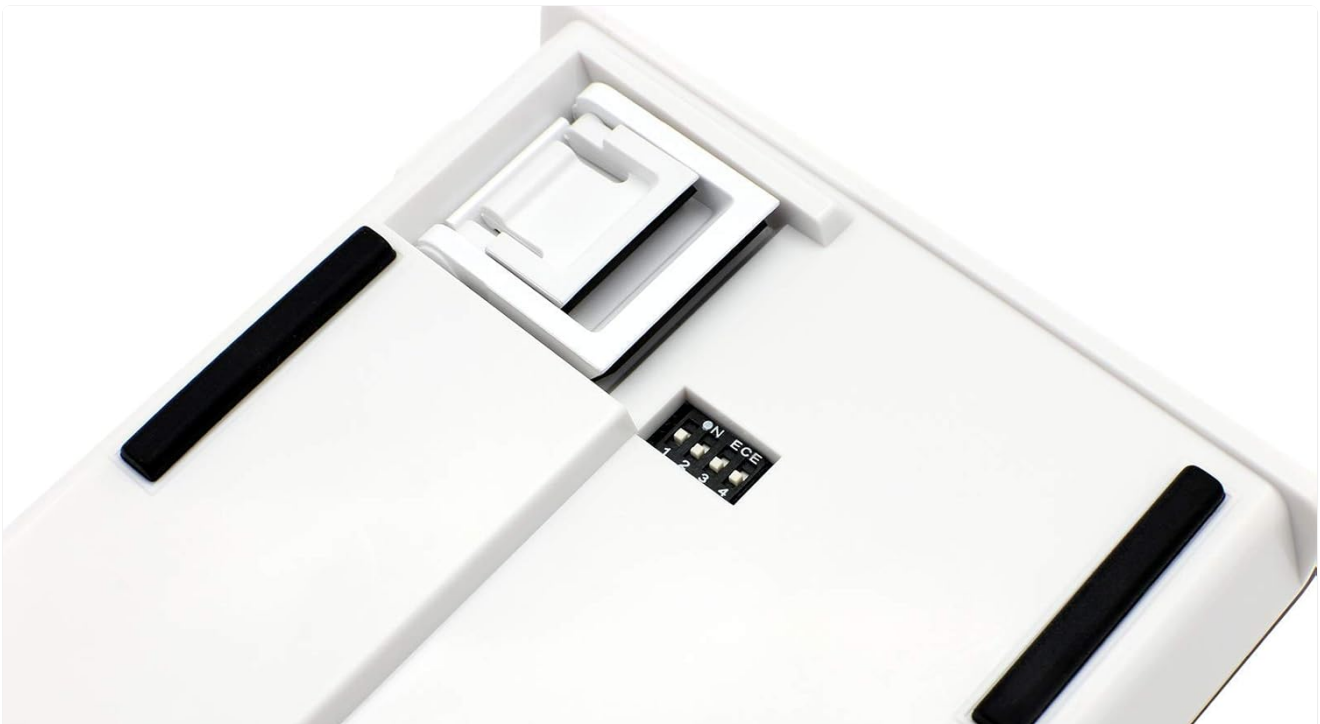
Image: A close-up of the underside of the Ducky One 2 Mini RGB keyboard, highlighting the DIP switches for advanced configuration.
