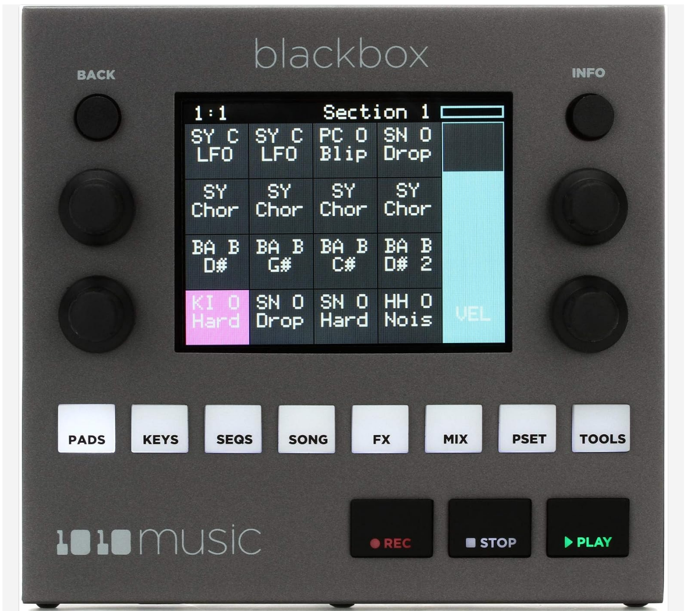
Figure 1: Front view of the 1010music Blackbox Studio, showcasing its central touchscreen display, rotary encoders, and control buttons. The screen displays a grid-based interface for sample and sequence management. Below the screen are navigation buttons labeled PADS, KEYS, SEQS, SONG, FX, MIX, PSET, and TOOLS. At the bottom, there are dedicated REC, STOP, and PLAY transport controls.
