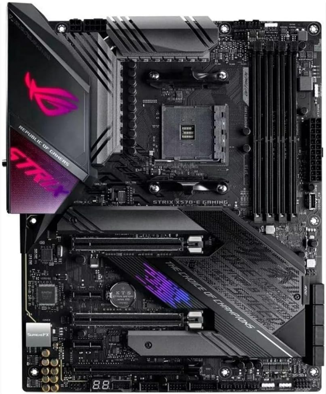
Figure 1: Top-down view of the ASUS ROG Strix X570-E Gaming Motherboard, highlighting the CPU socket, DIMM slots, and heatsinks.
