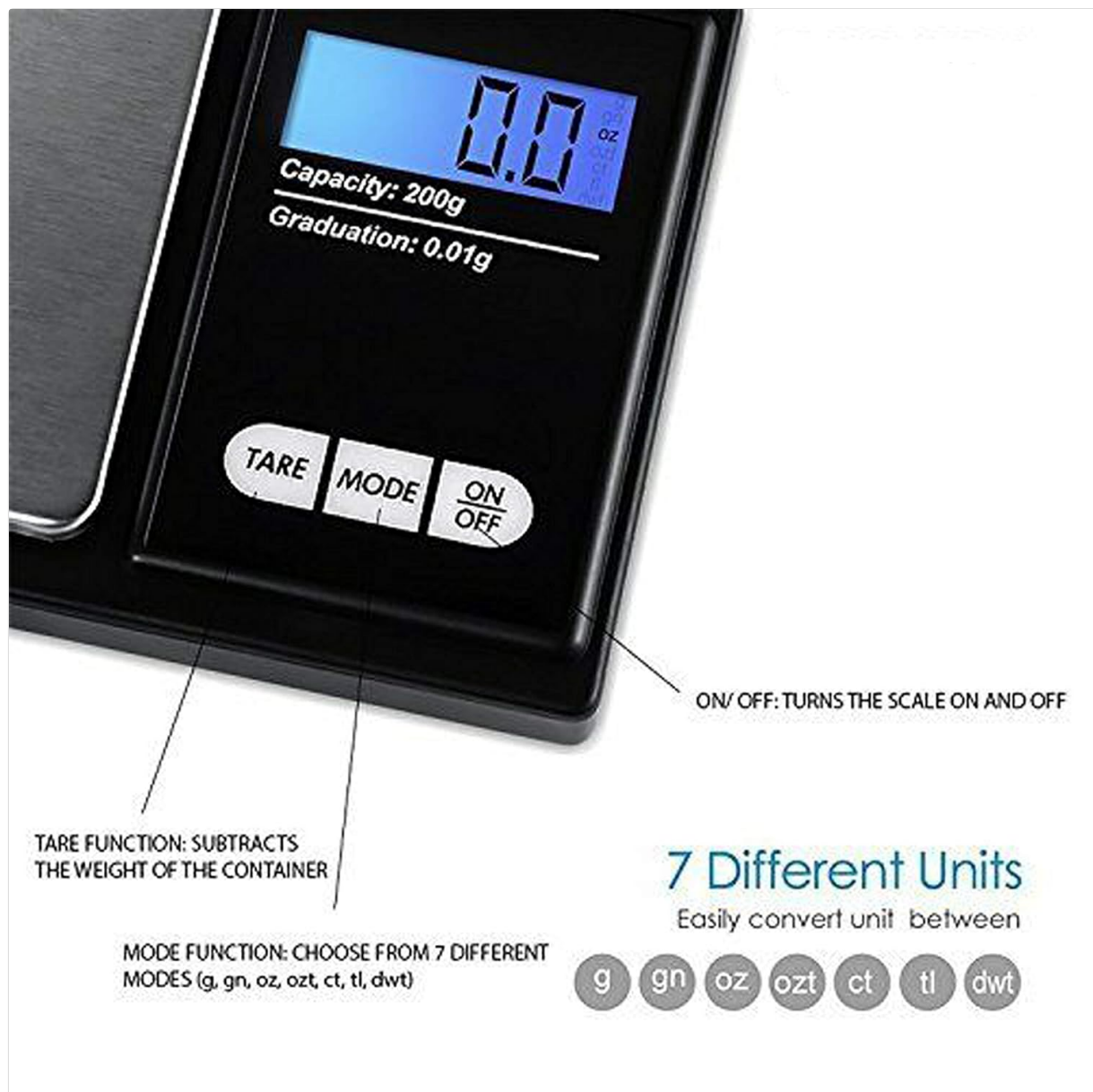
Figure 4.2: Available weighing units and button functions.
