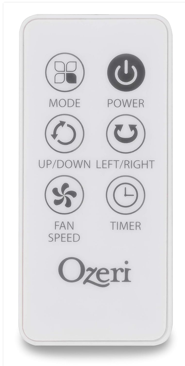
Figure 4.3: The remote control for the Ozeri 360 Duo Tower Fan. It features buttons mirroring the main control panel for convenient operation.
