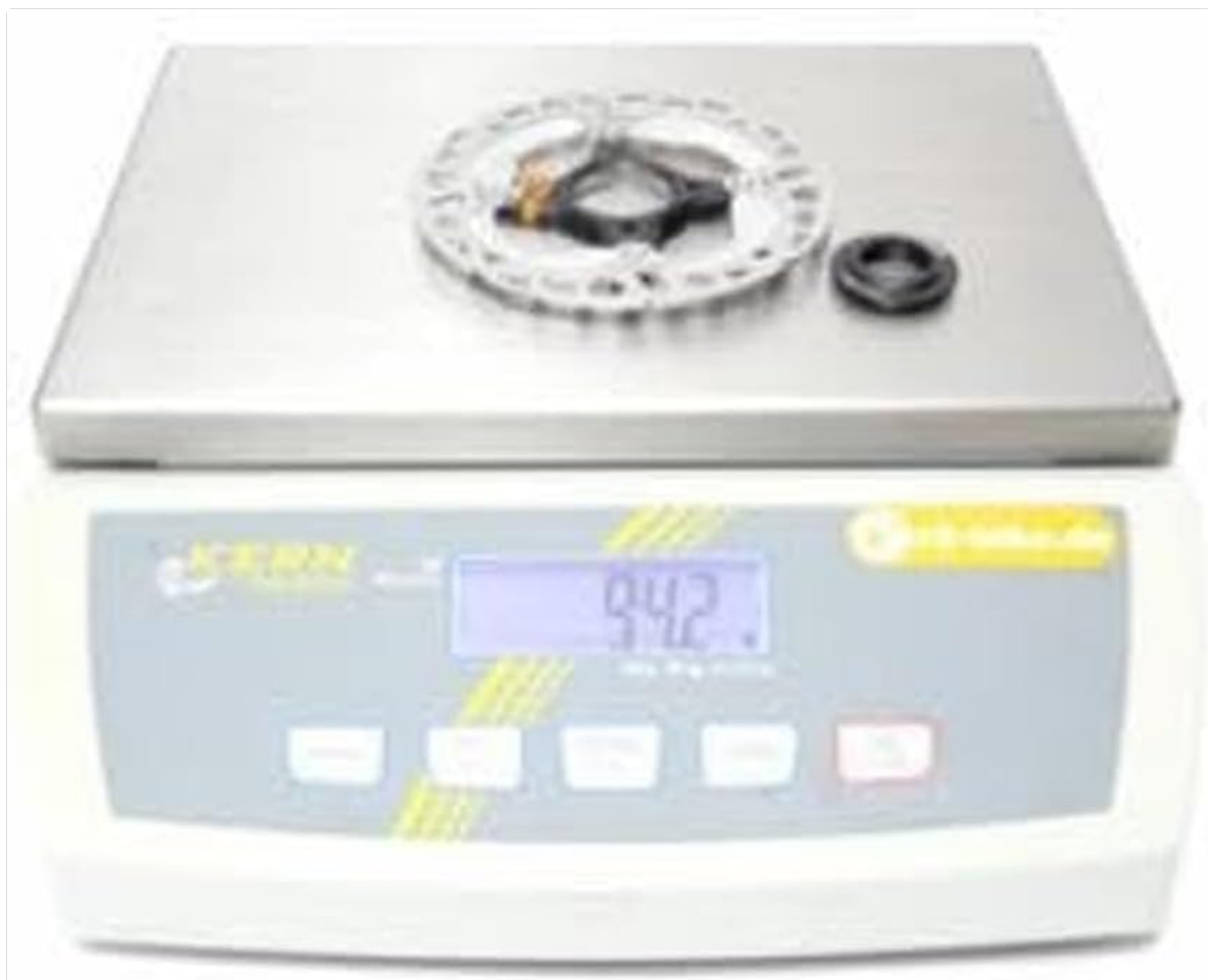
Figure 2: The SHIMANO RT-MT800 Disc Brake Rotor being weighed, illustrating its lightweight design. Regular inspection includes checking for wear and ensuring it meets minimum thickness specifications.
