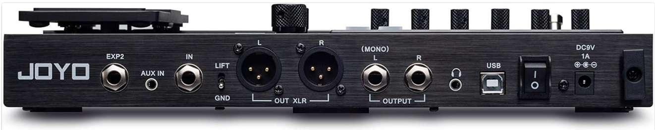
Figure 3: Detailed view of the rear panel, showing various input/output ports including EXP2, AUX IN, IN, OUT XLR, OUTPUT, USB, and DC9V.
