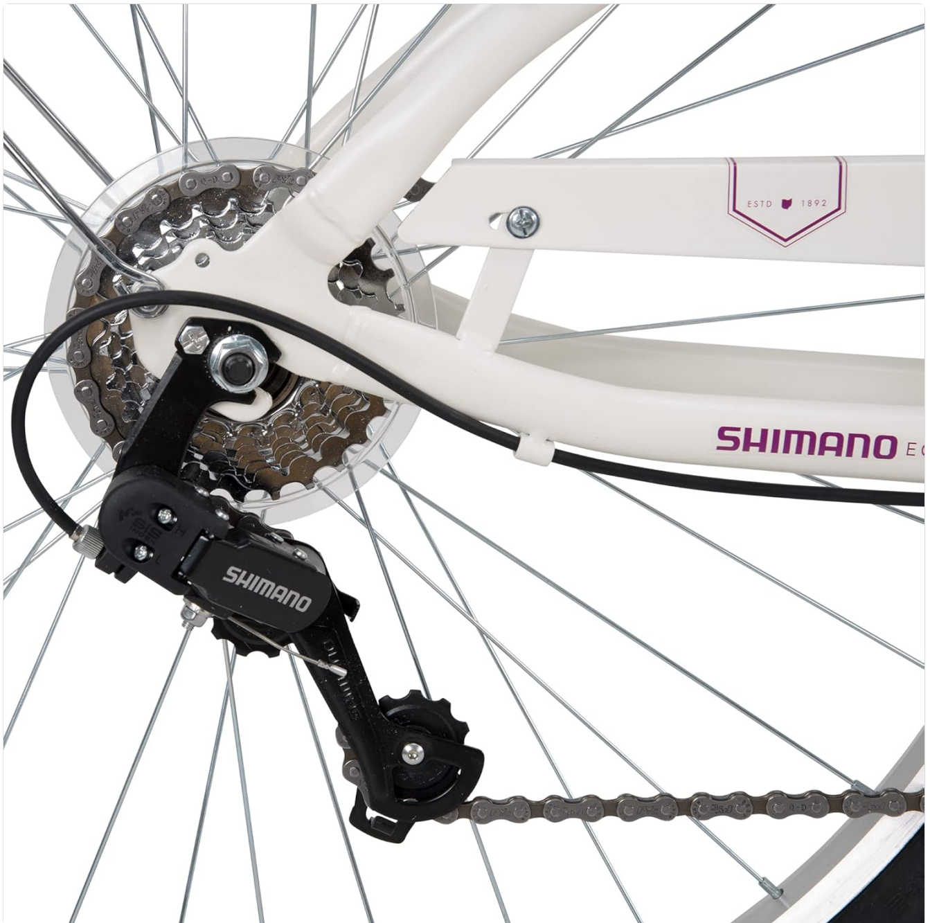
Image: A close-up view of the SHIMANO rear derailleur and cassette, part of the 7-speed system.
