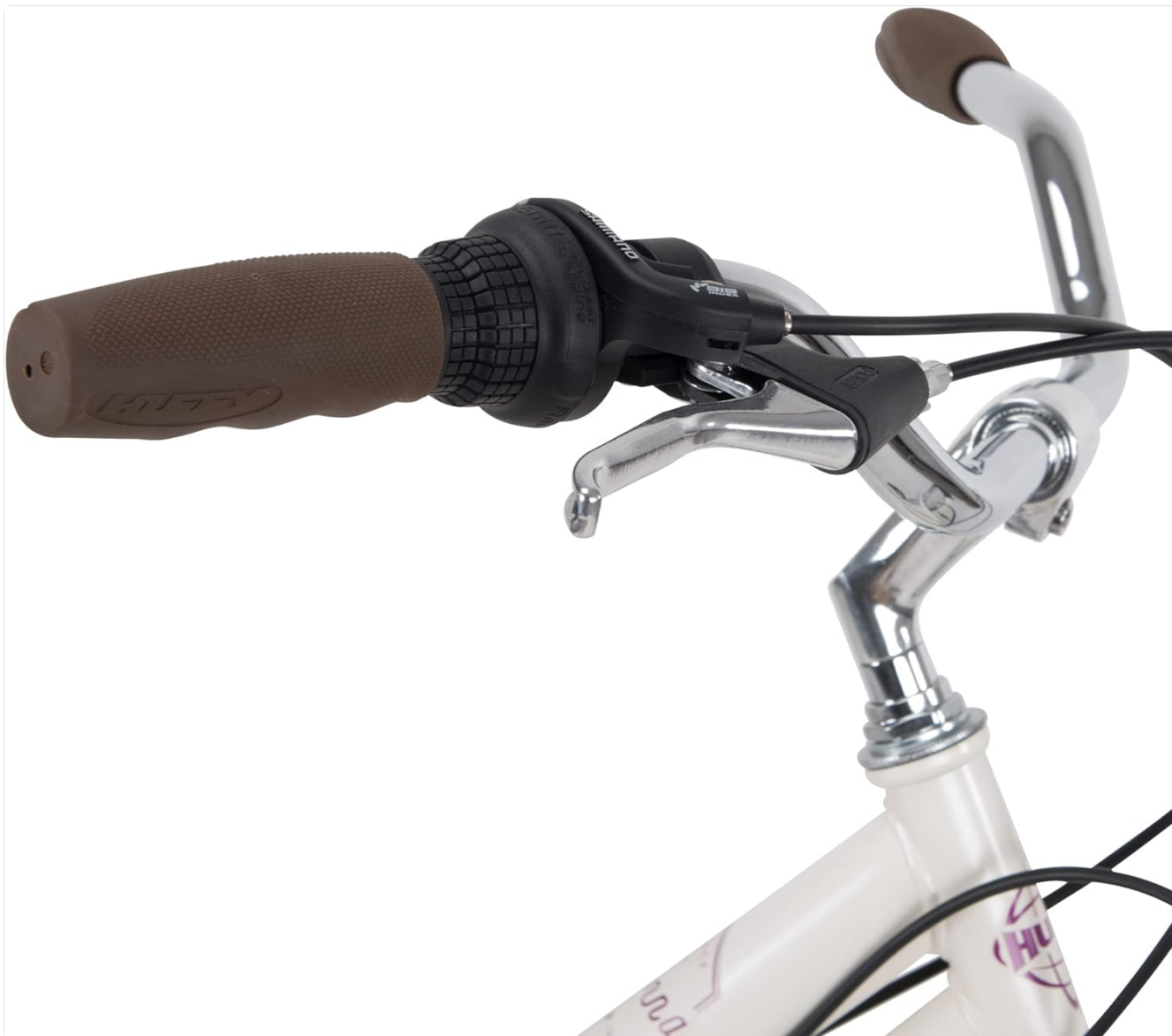
Image: Detail of the handlebars, showing the SHIMANO Revoshift gear shifter and brake levers.
