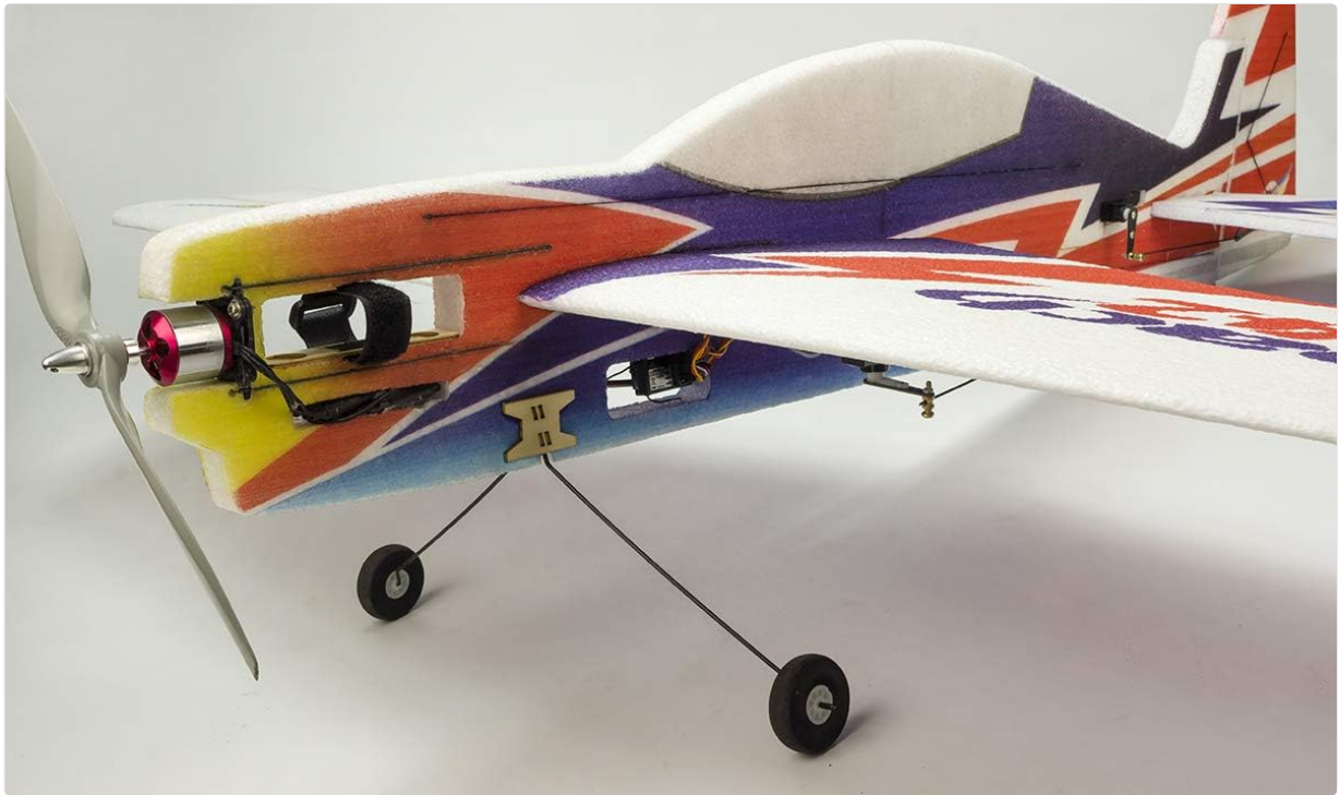
Image: Close-up of the motor and propeller assembly on the aircraft's nose.
