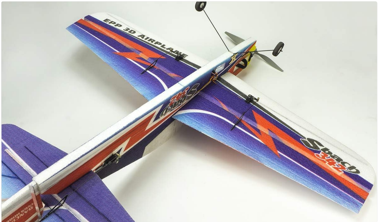
Image: Servos installed in the wing, connected to control surfaces.
