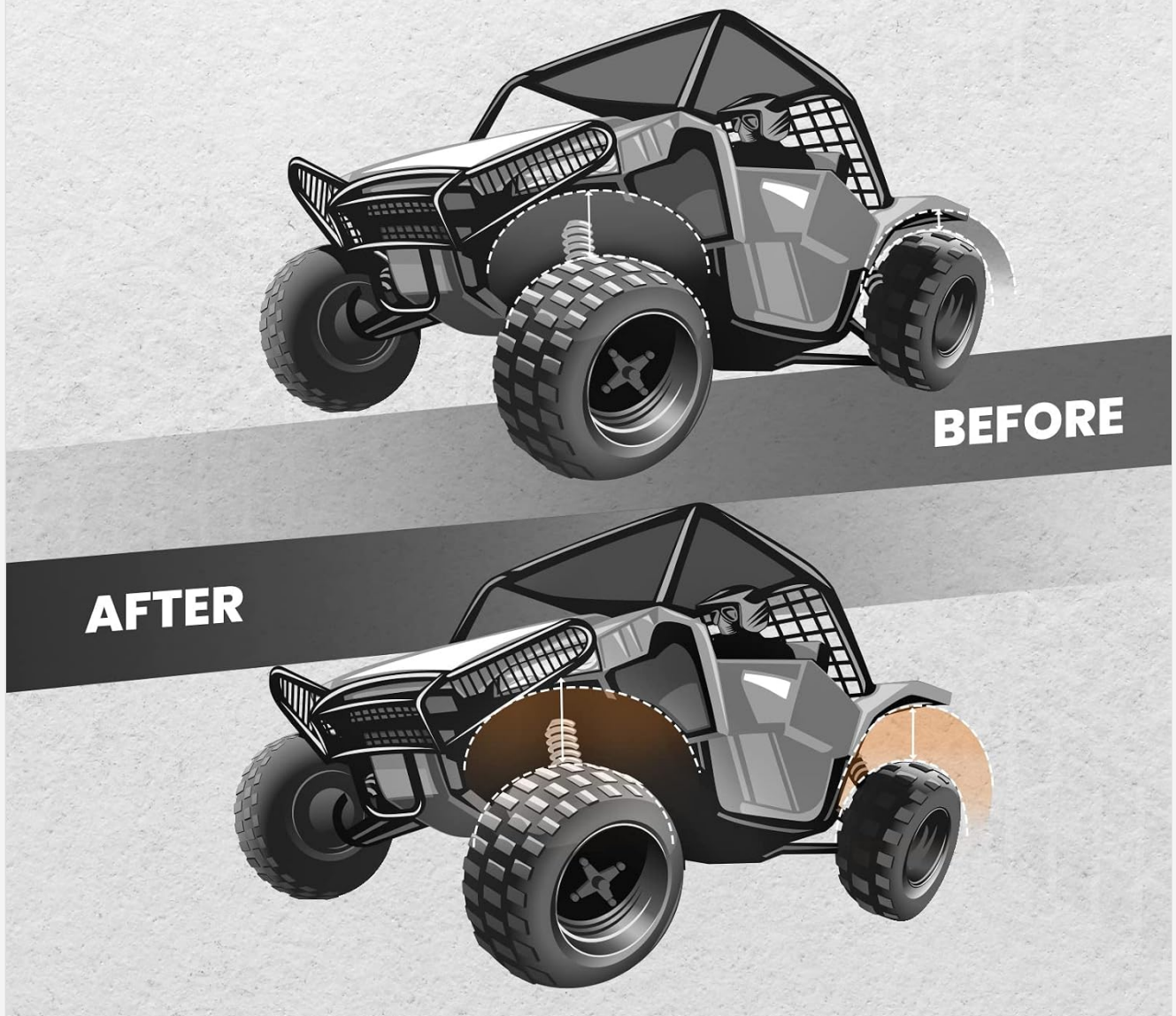
Image 6.2: Conceptual diagram illustrating the increased ground clearance (2 inches front and rear) achieved after installing the lift kit.
