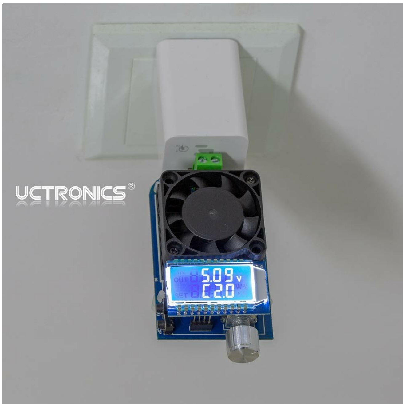
Figure 4.2: The load tester connected to a wall charger, used for evaluating charger performance.
