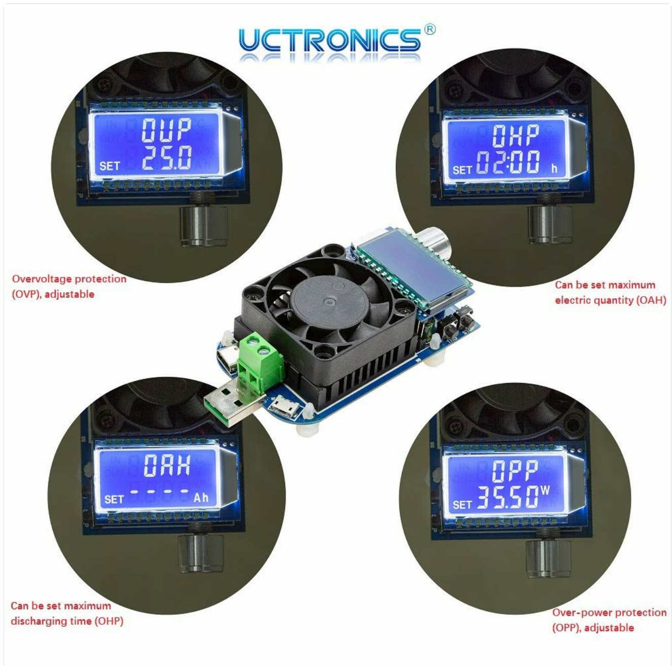
Figure 5.1: The LCD display showing adjustable protection settings for safe operation.
