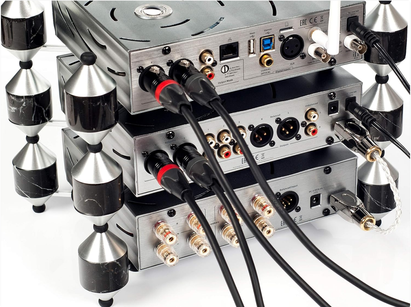
Figure 5: Example of a stacked iFi Pro system, illustrating rear panel connections for multiple units.
