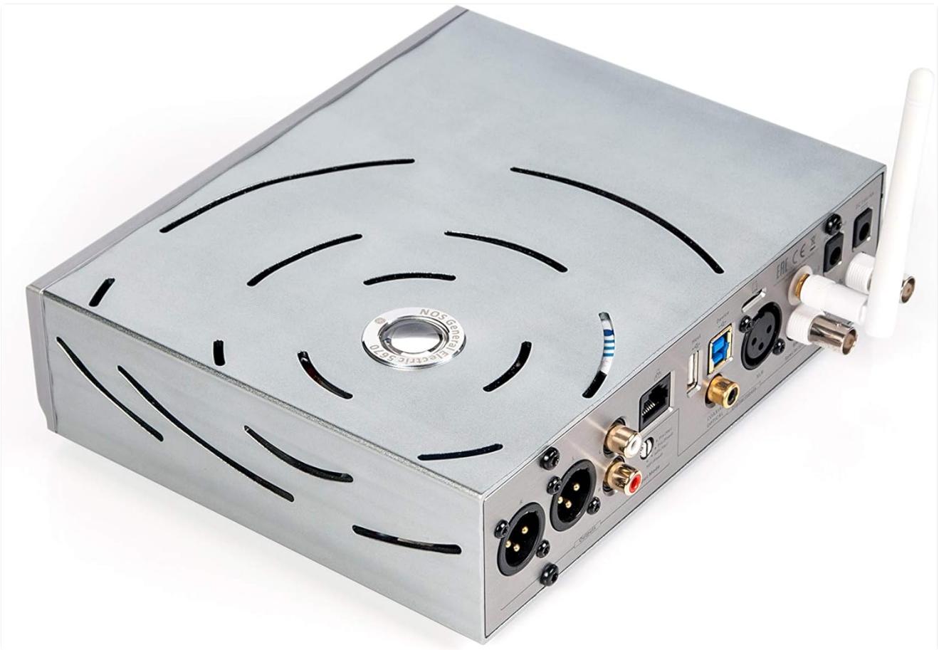
Figure 4: Rear panel connections of the Pro iDSD, including balanced XLR, RCA, Ethernet, USB Type A and B, digital inputs (Coaxial, Optical, AES/EBU, BNC), Micro SD slot, and power input.
