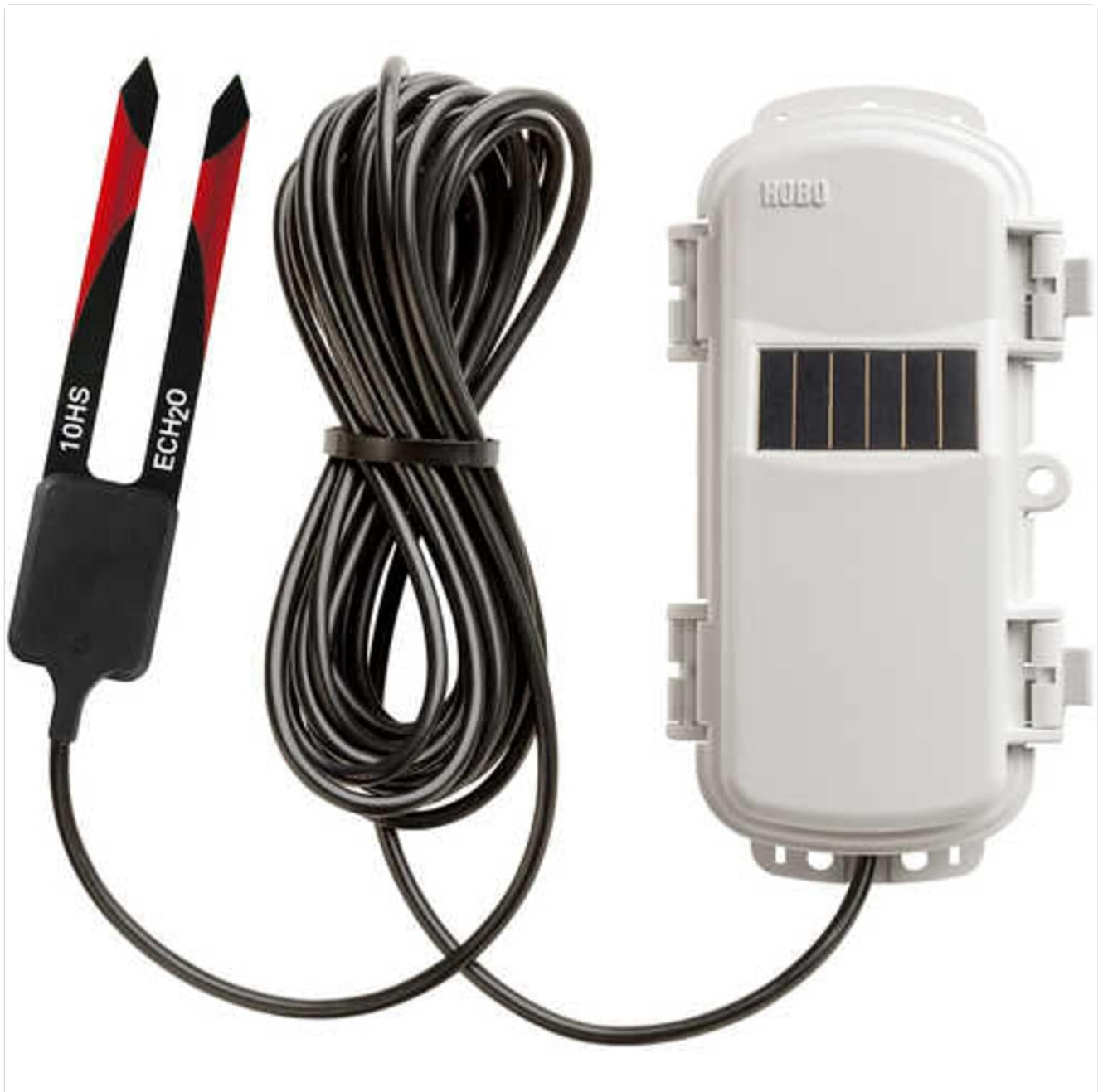
Figure 1: The Onset RXW-SMD-900 HOBOnet Wireless Soil Moisture 10HS Sensor. This image displays the soil moisture probe with its two prongs, connected by a cable to the wireless mote, which features a solar panel for power.
