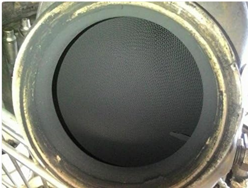
Image 5.1: Example of a DPF before cleaning, showing heavy soot accumulation.
