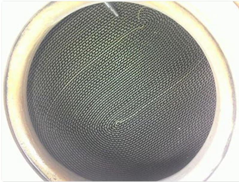
Image 5.2: Example of a DPF after cleaning, showing clear honeycomb passages.
