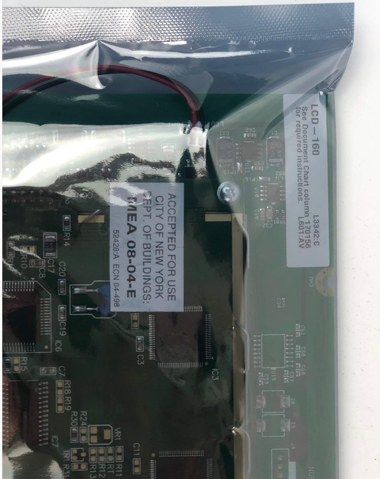
Image 2.5: A close-up view of a label on the LCD-160 circuit board, indicating model information and compliance details.
