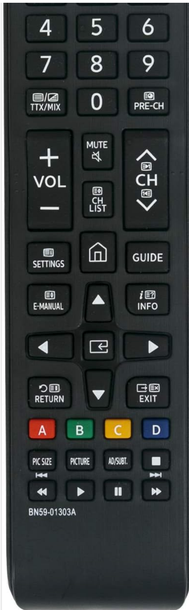
Figure 1: Front view of the BN59-01303A remote control. This image displays the full layout of the remote, including the red power button at the top left, a numerical keypad, volume and channel controls, directional navigation buttons, and dedicated function keys for various TV
