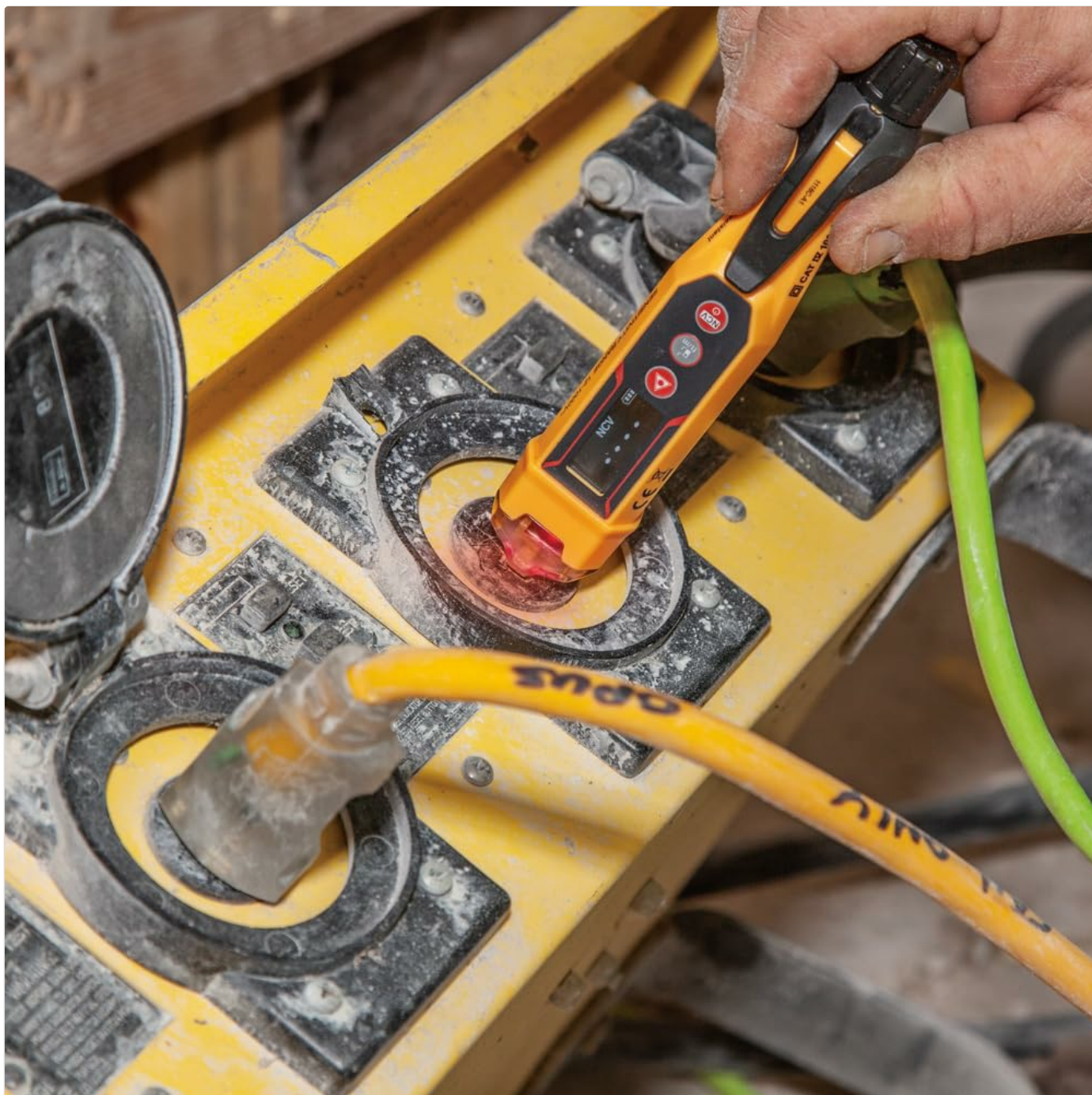
Figure 3: The NCVT-6 detecting voltage on a heavy-duty power strip, indicated by the red light.
