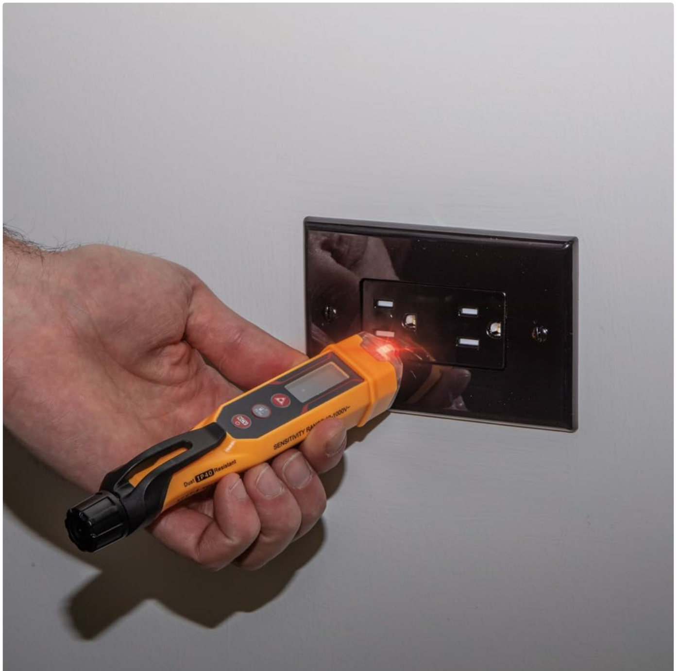
Figure 2: Using the NCVT function on a standard electrical outlet.
