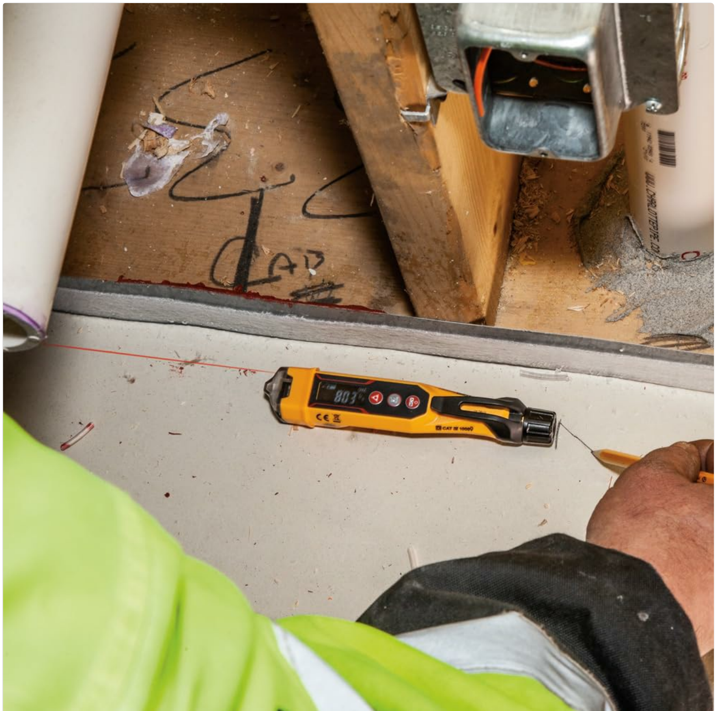
Figure 6: The laser distance meter function being used to measure a distance on a flat surface.
