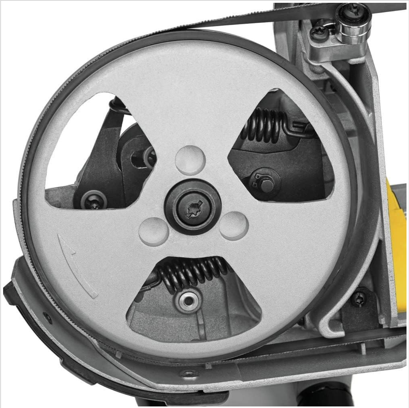
Figure 4: Internal view showing the blade path around the drive wheels and the tensioning components.
