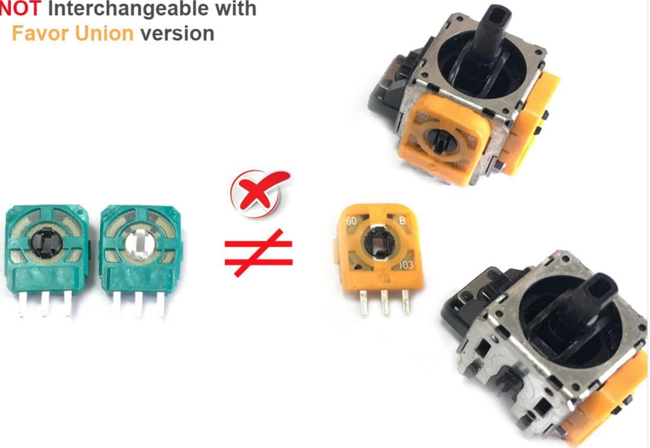
Figure 3: ALPS vs. Favor Union Potentiometer Compatibility. This image visually demonstrates that ALPS potentiometers (green) are not interchangeable with Favor Union potentiometers (orange), emphasizing the importance of using the correct type for your controller.
