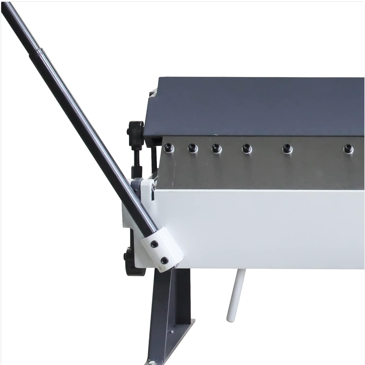
Image: Side view showing the installed operating handle and counterweight, essential for leverage during bending.
