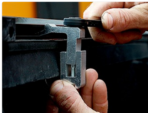
Image 4.3: An image showing hands adjusting the tension mechanism of the tonneau cover, which helps keep the vinyl taut and wrinkle-free.
